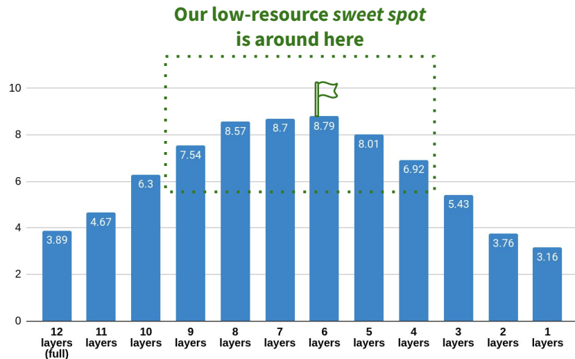
Figure: BLEU scores (dev) for AST Tamasheq-French models using different number of wav2vec 2.0 encoder layers (Tamasheq-only model)
